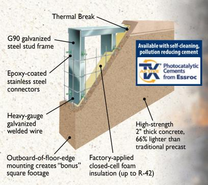
Architectural Precast Concrete/Steel Stud Building Panels
